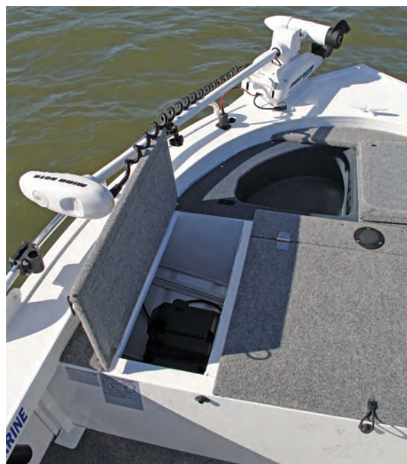
There's an anchor well forward and bolted to the bow is the latest 'electric' anchor – the Minn Kota RT55ST Terrova iPilot.
